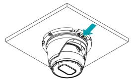
5 The top cover rotates on the bottom cover and is tightened.
