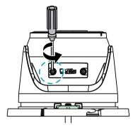
2 Insert a SD memory card into the SD memory card slot with the 'micro SD' print facing downward.
