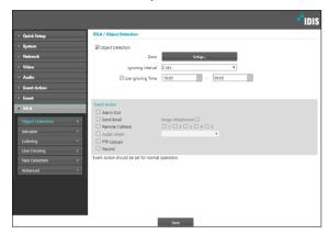
Zone: Click Setup and define the object detection area and the conditions for which an object detection event will occur in each area up to 8 conditions.
