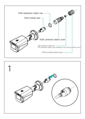
Insert a round rubber ring (silicone rubber) into the RJ45 jack.
