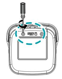
2 Insert a SD memory card into the SD memory card slot with the 'micro SD' print facing upward.
